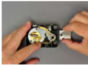
Holding the lever in place, and depressing the relock trigger arm as shown, remove the lock bolt.
