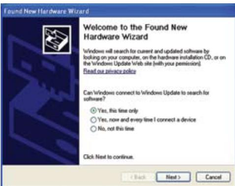
10. Windows will then find the newly connected USB reader, and will open the wizard that adds new hardware to the system. Follow the on-screen directions to enable your computer to recognize the new USB reader as a hardware device.
