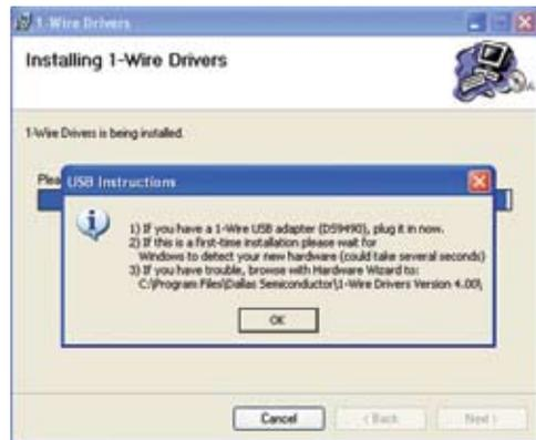
9. After some time, the installation routine will finish, and you will be prompted to connect the USB reader. Connect the reader to a USB port on the computer. **Do NOT connect the reader to a hub or docking station.**
