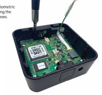
10. Slide the ribbon cable into the biometric connection.
