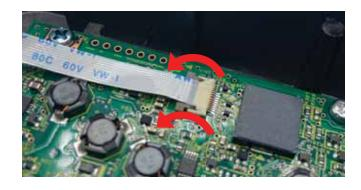
12. Check the ribbon cable to make sure the mounting of the keypad will not damage the cable.
