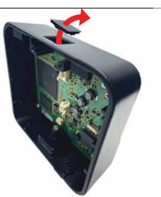
8. Slide the biometric sensor into the keypad housing ensuring the biometric ribbon is moving towards the right and over the green ground cable.
