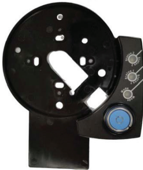
Keypad Extension Base Installed under the keypad. This is required when using the lock's Service Mode. The extension base provides a green LED to indicate "Status 1", and a red LED to indicate "Status 2" and a yellow LED to indicate "Mode" of lock operation. The extension base also provides a port for communication with Touch Keys.
