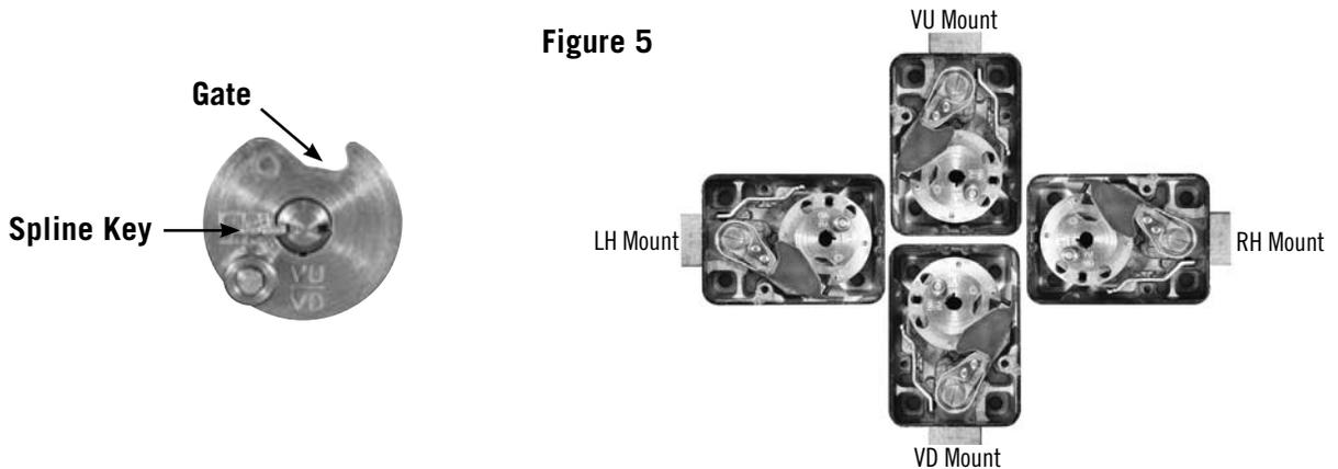
12. Insert the spline key with the tip toward the edge of the cam. Tap in lightly. Be very careful to avoid striking the stainless steel roller that is attached to the top surface of the drive cam. With the spline key inserted fully, the dial must turn freely with no rubbing or interference.
