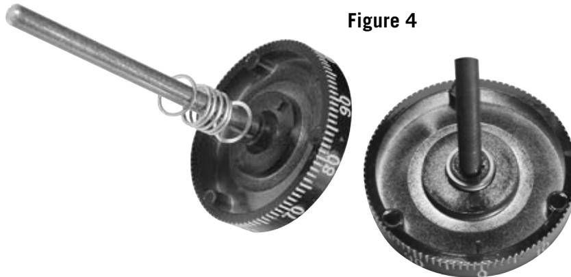
10. Insert the dial into the lock, but remember that you should not allow the cam to slide outward against the accelerator spring, possibly damaging it. Hold the drive cam in place, positioned for its gate to receive the nose of the drop lever, and thread the dial into the cam until the dial stops.
