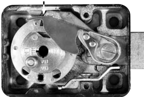
Accelerator Spring in Loaded Position
