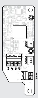
Requirements: Operating Voltage 12-24 VDC Conductors 18-22 AWG
