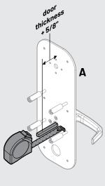
Cut exterior spindle where marked, use metal file to smooth edges. After cutting, insert exterior spindle into handle drive hole.
