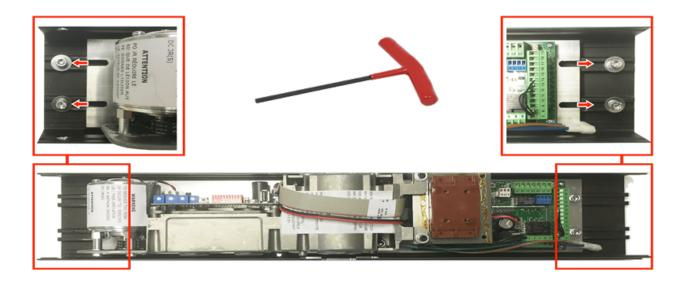
Next, locate & loosen the 4 side hex bolts (see above) using a 5mm allen wrench.
