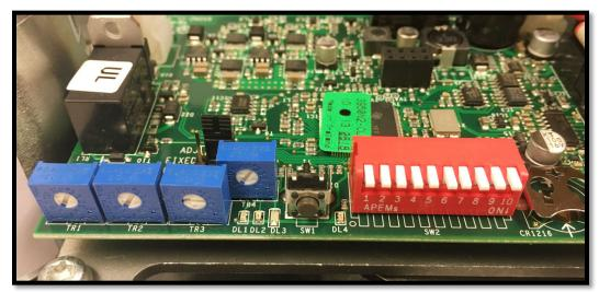
applications, and with DIP #2 ON for pull applications. All other dip switches may be set after the initial setup.
