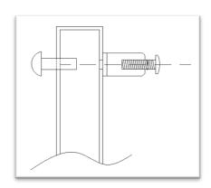
When attaching the header to the hollow metal door frame, ensure there are 5 attaching screws spaced equally apart. They should be #12 sheet metal type screws.
