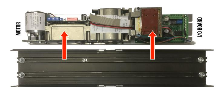
Remove the drive plate by shifting the drive plate to the left and lifting the drive plate away from the back plate.
