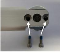
Then, horizontally slide the adaptor onto the primary arm until the two mounting holes of spindle line up with the corresponding holes on the primary arm. The spindle is intended to fit tightly. Secure the spindle using the two small hex bolts, **BUT DO NOT OVERTIGHTEN**.
