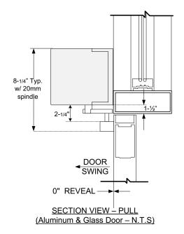
PULL ARM APPLICATIONS: Bottom of operator is mounted 1.5" up from the bottom side of top door frame
