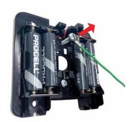
7. Remove the plastic biometric insert at the top of the keypad by pressing upward from the inside of the keypad housing.
